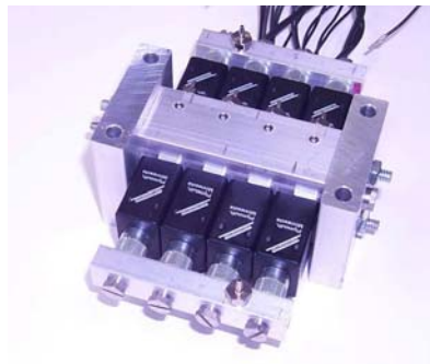
Modular block of four valves
