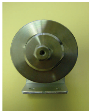
Assembled filter with 1/8" Swagelok fittings
